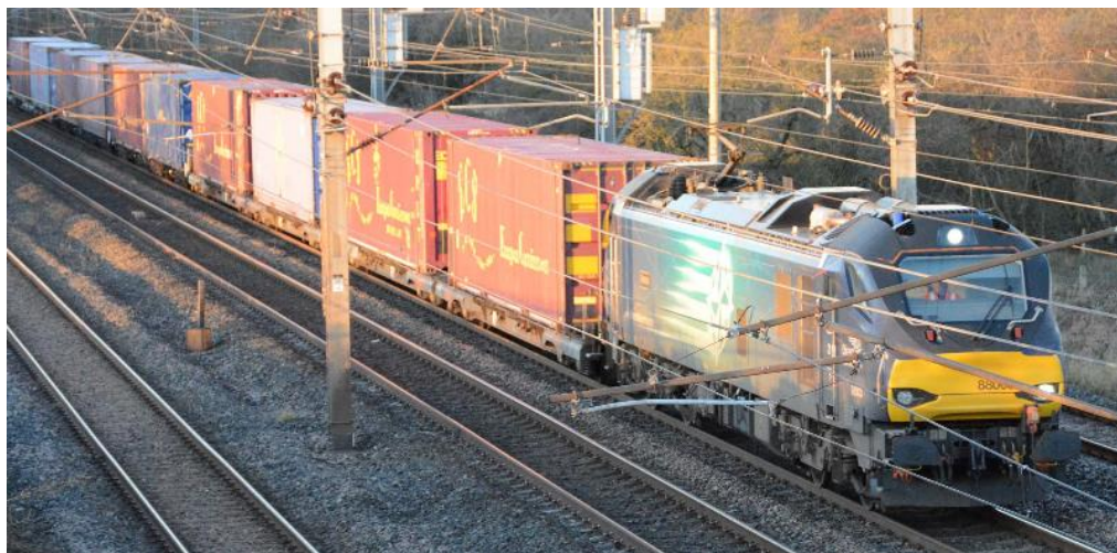
DRS Class 88 can operate on electric or (at reduced power) on diesel
